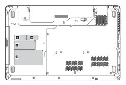
For some models, you also need to apply one or two FCC labels. Check the old base cover; if it has one or two FCC labels, find duplicates of them in the label kit and apply them to the new base cover.
